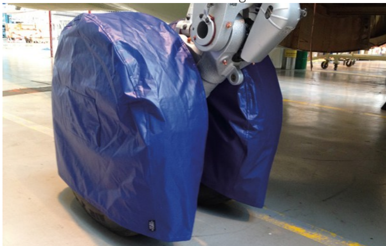
Figure 546. Protect Tires From Contaminants
