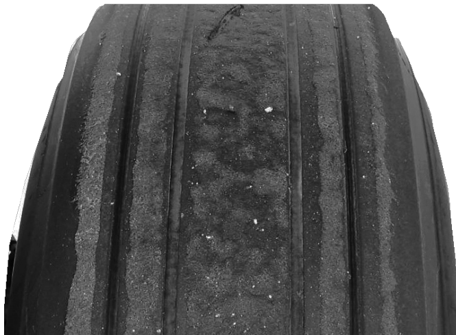
Figure 547. Contamination From Hydrocarbons
