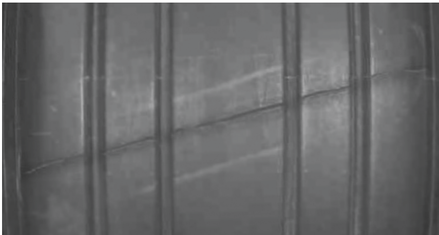
Figure 531. Open Tread Splice
