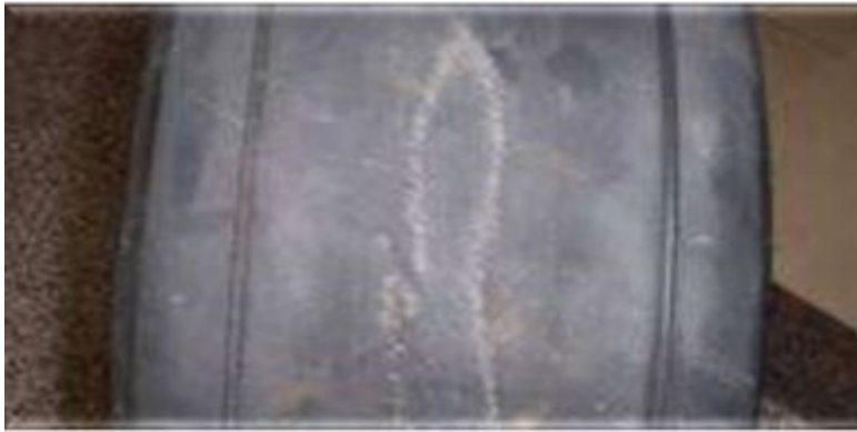
Figure 513. Center Wear (Overinflated)
