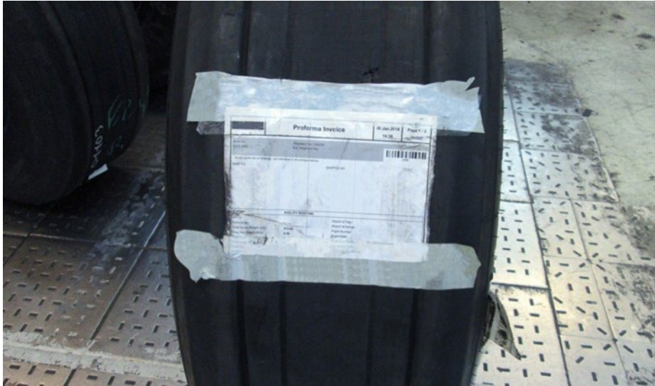
Figure 614. Recommended Placement of Adhesive Labels on Tires
