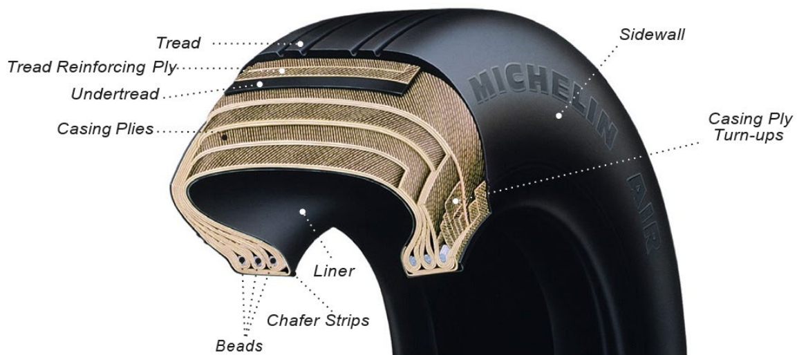
Figure 103. Bias Aircraft Tire
