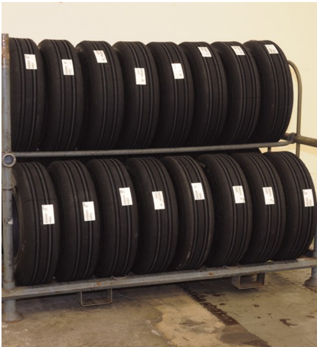
Figure 305. Store Tires Vertically in Racks (Left). Tires Stacked Horizontally (Too many tires) (Right)
