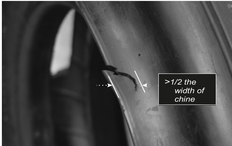
Figure 538. Damage to Chine Tire
